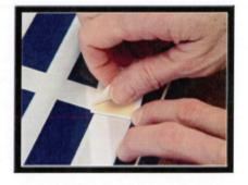
4) Align left and bottom of record plate with left and bottom of guide box on record board.
